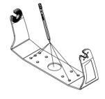
4: Remove the display unit and use the mounting bracket as a template to mark the four positions of the screw holes and optional center cable hole.
